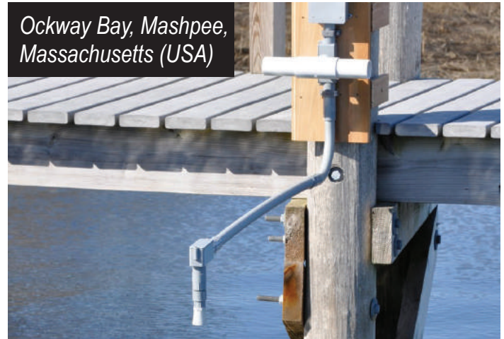
Tide level measurement is a common use for the MaxSonar sensor and the ioBridge IO-204. Connecting the MaxSonar sensor to the ioBridge IO-204 module is a simple-to-use wireless or remote sensing interface for monitoring measurements to a target from anywhere in world. In this application the community must monitor tide levels because they will not be able to enter the bay when tide levels are low.
