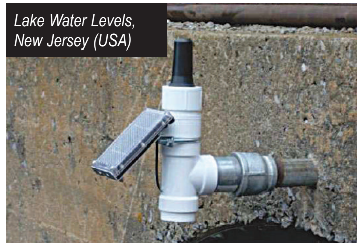
The MaxSonar sensor is integrated into a wireless solar power system for monitoring lake water levels. The MaxSonar sensor survived and was operational after Hurricane Sandy hit the shores of New Jersey in October 2012. The customer comments: "The system has completed several months of trials under harsh conditions. The solid performance of the MaxBotix sensor has us confident in the system performance, and we are now ready to take the system live to the community!"
